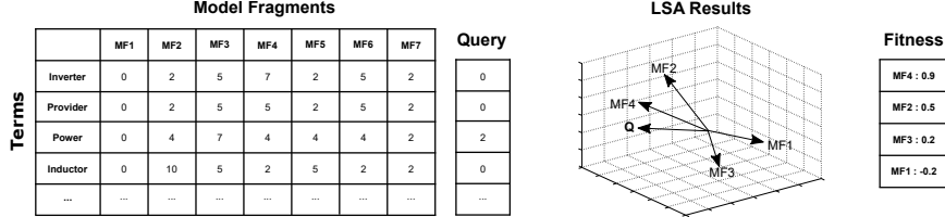
Fig. 4. Fitness Operation via Latent Semantic Analysis (LSA) - term-by-document co-occurrence matrix (left) and vector representation (right)
