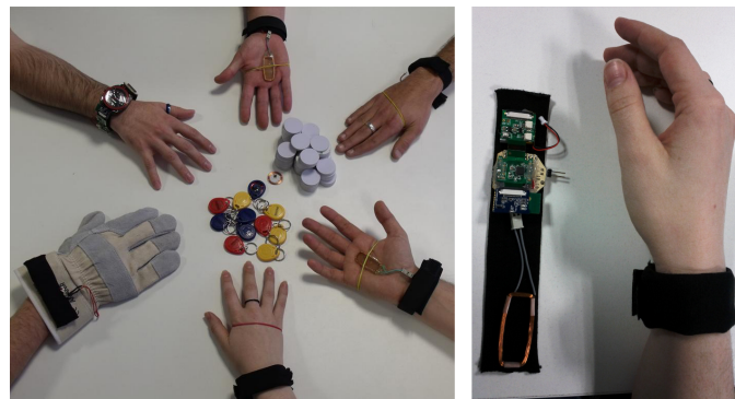
Figure 2. Different prototypes of our RFID Tag reader, such as a glove, a bracelet and a watch (left). The final prototype used in our evaluations (right).
